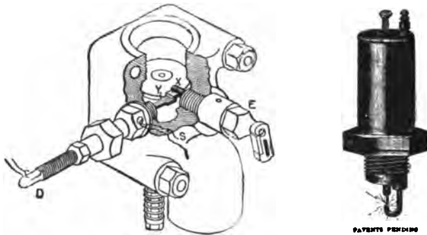
FIG. 327. —Details of a Common Form of Contact for Producing a Wiping Spark. The electrode, X, rotated by the crank, E, as indicated, gives a wiping contact and break at the terminal, Y, which is tipped by a resilient platinum spring. One of the wires forming the circuit is connected at D through the insulated plug screwed into the body of the ignition chamber; the other is connected to the metal of the chamber at the nut, M. The advantage of this form of sparking device is that the constant contact of the electrode keeps the surfaces clean, but at the same time the constant friction produces an immense wear for the same reason. An excellent form of simple make and break device is shown in connection with the suction of the Duryea cylinder in a succeeding chapter.
